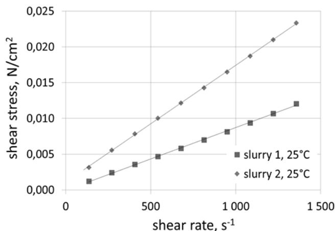
Fig. 5. Influence of the shear rate on the shearing stresses of the liquid ceramic slurries 1 and 2 at a temperature of 25°C
