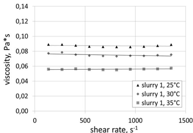
Fig. 8. Influence of the shear rate on the dynamic viscosity of the liquid ceramic slurry 1, prepared on the basis of the water binder Ludox AM, at temperatures: 25, 30 and 35°C
