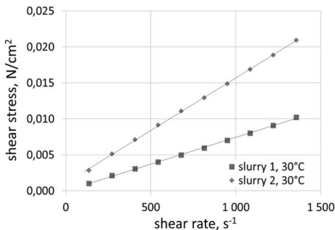
Fig. 6. Influence of the shear rate on the shearing stresses of the liquid ceramic slurries 1 and 2 at a temperature of 30°C
