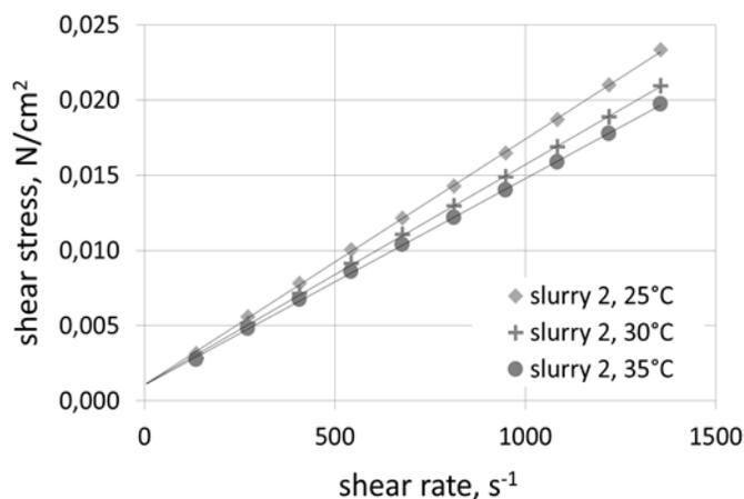
Fig. 4. Influence of the shear rate on shearing stresses of the liquid ceramic slurry 2, made on the basis of the water binder Ludox AM at a temperature: 25, 30 and 35°C
