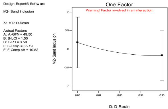
Fig. 7. Resin as a single variable for sand inclusion defect at a stated design point
