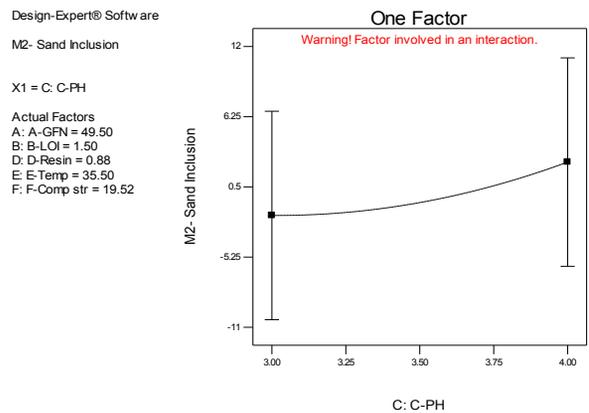
Fig. 8. pH as a single variable for sand inclusion defect at a stated design point
