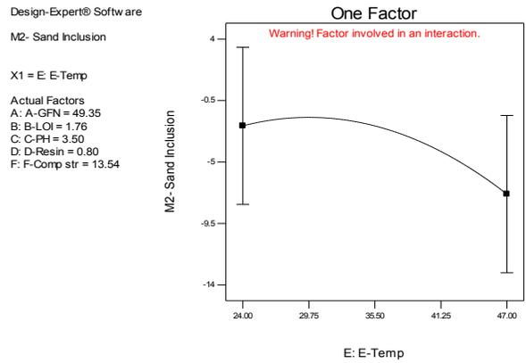
Fig. 6. Sand Temperature as a single variable for sand inclusion defect at a stated design point
