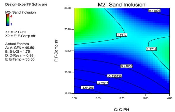
Fig. 13. Compressive Strength and PH level for sand inclusion defect at a stated design point
