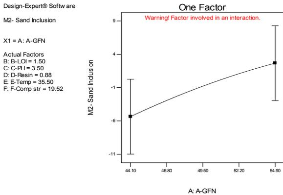
Fig. 9. GFN as a single variable for sand inclusion defect at a stated design point
