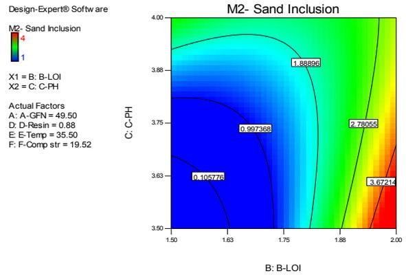
Fig. 11. Ph and LOI level for sand inclusion defect at a stated design point
