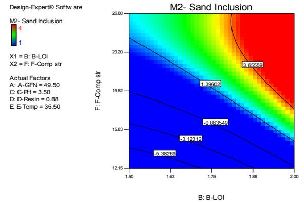
Fig. 12. Compressive Strength and LOI level for sand inclusion defect at a stated design point
