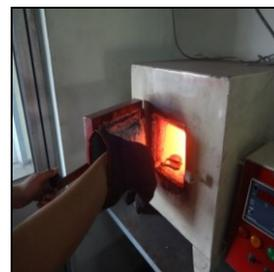
Fig. 2. LOI test performed at Krislur Castomech. Pvt. Ltd.
