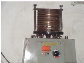
Fig. 1. Standard sieve test equipment
