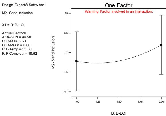
Fig. 10. LOI as a single variable for sand inclusion defect at a stated design point
