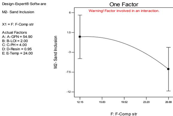
Fig. 5. Compressive strength as a single variable for sand inclusion defect at a stated design point
