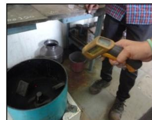
Fig. 4. Laser gun to measure temperature of sand
