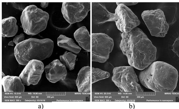
Fig. 7. Microscopic view of grains used silica sands
