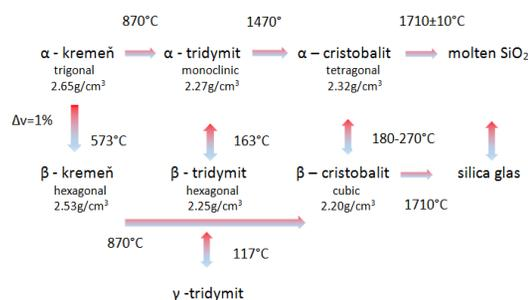
Fig. 3. Mechanism of polymorphic transformations SiO<sub>2</sub>
