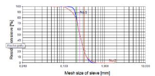
Fig. 8. Cumulative curve using silica sands
