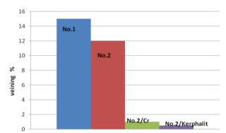
Fig. 4. Appearance veining on surface of cats in varying configurations of the core mixture
