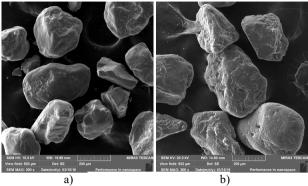
Fig. 7. Microscopic view of grains used silica sands a) No.1, b) No.2
