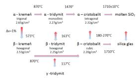
Fig. 3. Mechanism of polymorphic transformations SiO<sub>2</sub>
