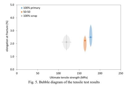
When tensile properties of all three conditions are compared, there was an interesting observation. As seen in the bubble diagram in Fig 5, as the scrap ratio was increased, ultimate tensile strength decreased (the x-axis values). However, elongation at fracture values for 100% scrap and 50-50% mixture appears to be
