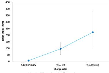
Fig. 4. Bifilm index of different charges
