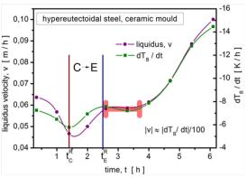
Fig. 6. Velocity of the liquidus isotherm movement; v
