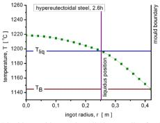
Fig. 5b. Liquidus position on the roll / ingot radius for the 2.6 [h] of solidification
