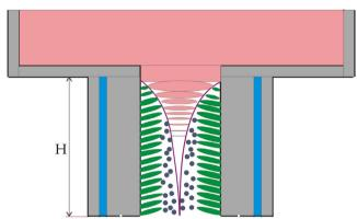
Fig. 9b. Formation of the columnar and equiaxed grains with the CET during the continuously cast brass ingots; the white point at the scheme bottom is the **operating point** to study / measure thermal behavior of the mold, Fig. 10b.
