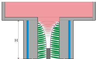
Fig. 9c. Formation of the columnar grains followed by a single crystal growth during the continuously cast brass ingots; the white point at the scheme bottom is the **operating point** to study / measure thermal behavior of the mold, Fig. 10c.
