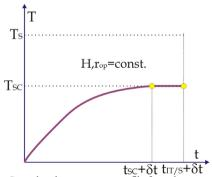
Fig. 10c. Speculated temperature profile for columnar structure formation completed by the single crystal growth
