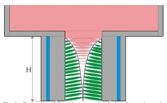
Fig. 9a. Formation of the columnar grains during the continuously cast brass ingots; the white point at the scheme bottom is the **operating point** to study / measure thermal behavior of the mold, especially, during the initial transient solidification, Fig. 10a.
