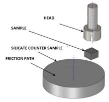
Fig. 5. Diagram of the steel and silicate counter-sample
