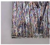
Fig. 2. Surface of the sample upon grinding
