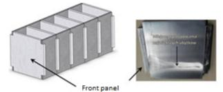
Fig. 1. Matrix for producing a silicate brick; worn front panel
