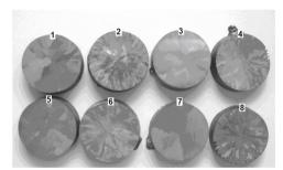
Fig. 3. Macrostructure on cross-sections of castings
