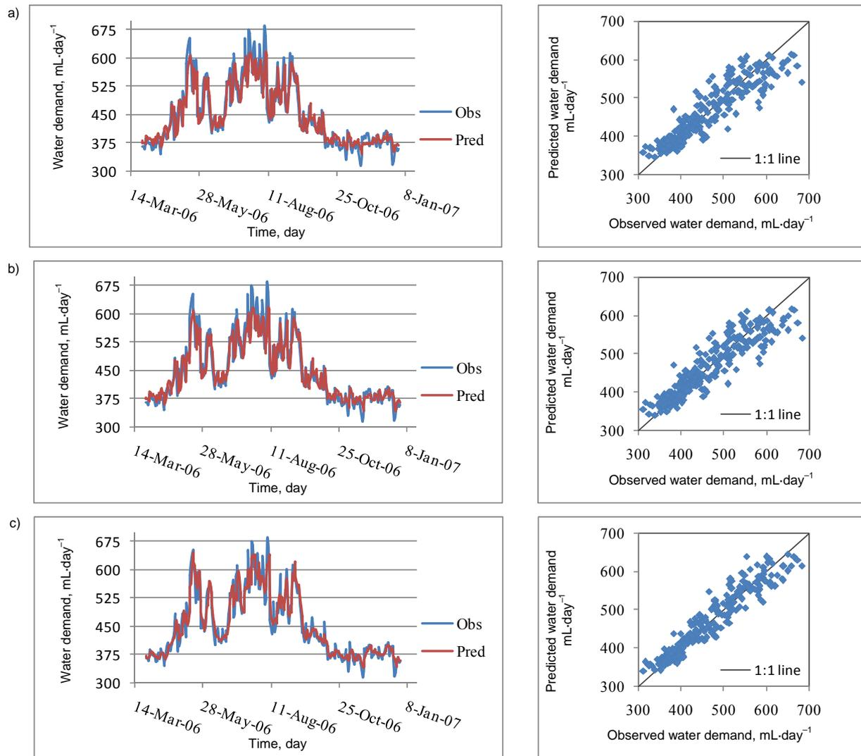
Fig. 3. Hydrographs and scatter plots for observed (Obs) and predicted (Pred) water demand in Calgary for 1 day lead time forecasts for the testing dataset using the best models: a) ELM, b) B-ELM, c) W-ELM; source: own study
