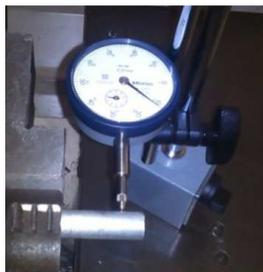
Fig. 16. Runout measurement using a dial indicator.
