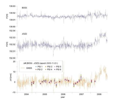
Fig. 9. Comparison of relative deformations in height component between Borowa Gora and Jozefoslaw obtained from GNSS (daily solutions) and PSI data
