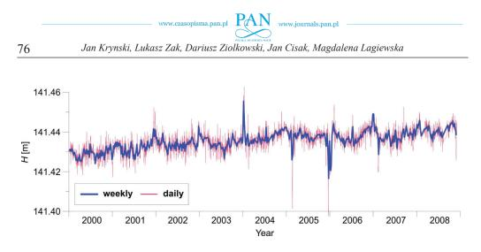
Fig. 1. Example of height variations of JOZE station from daily and weekly solutions of the short vector BOGO – JOZE with the reference station BOGO
