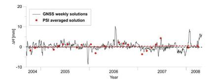
Fig. 10. Comparison of relative deformations in LOS component between Borowa Gora and Jozefoslaw obtained from GNSS (weekly solutions) and PSI (average) data
