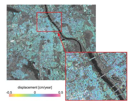
Fig. 3. The example of deformation map obtained as a result of processing radar images with the use of the PSI method
