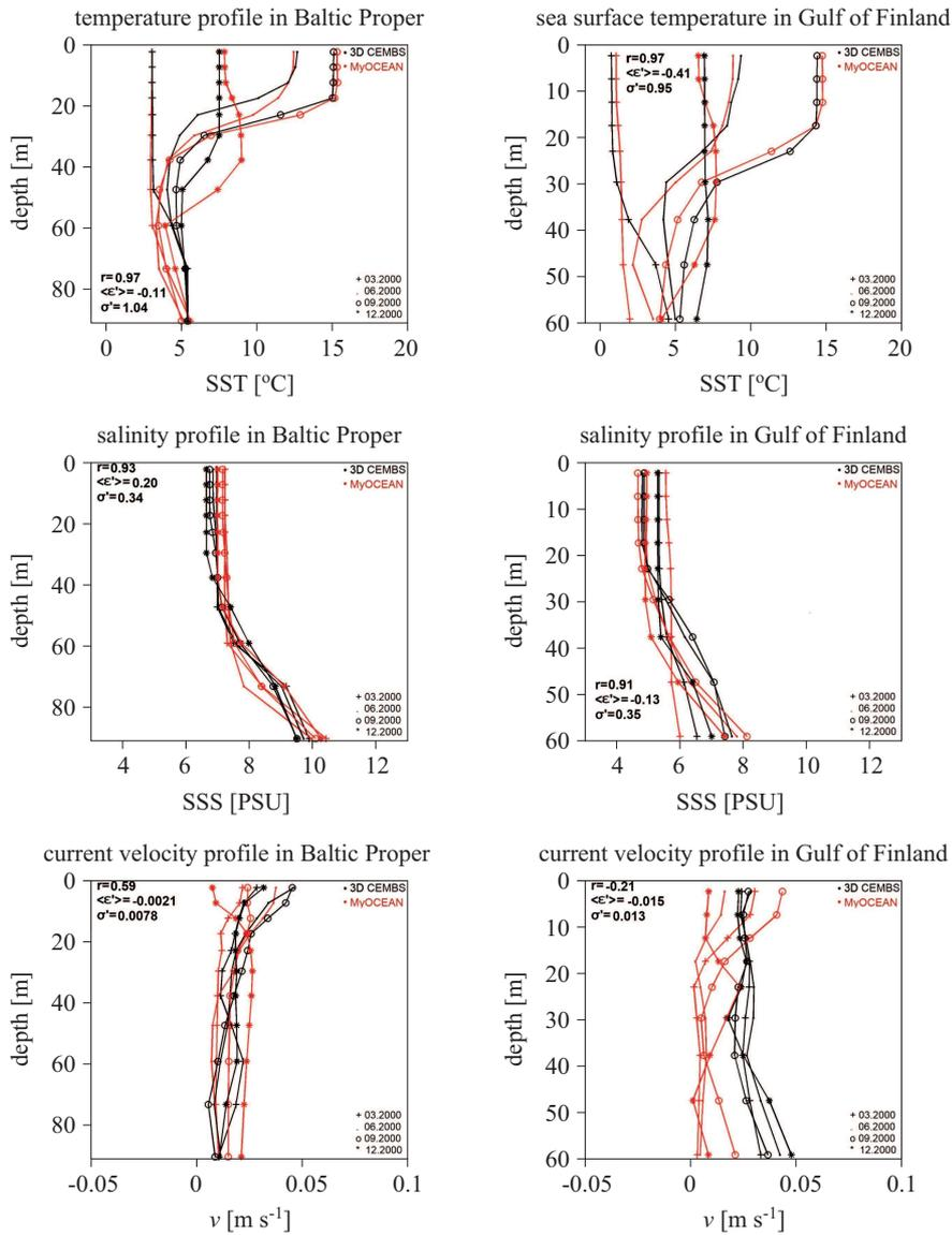
**Figure 8.** Data from MyOcean and 3D CEMBS model. Vertical profiles of the main hydrodynamic parameters, temperature, salinity and velocity (absolute value) for two regions (Baltic Proper and Gulf of Finland)
