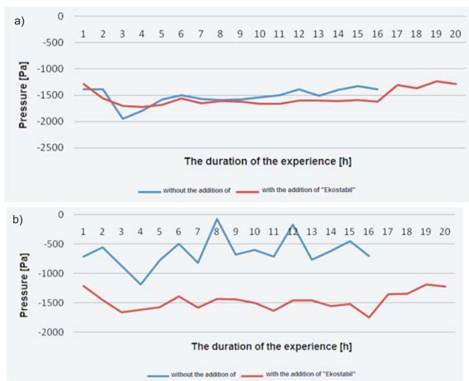
Figure 5. Pressure change in the pipe precipitation, during two measurement series, with and without EKOSTABIL, above the siphon: a) 1.25 m, b) 0.95 m.
