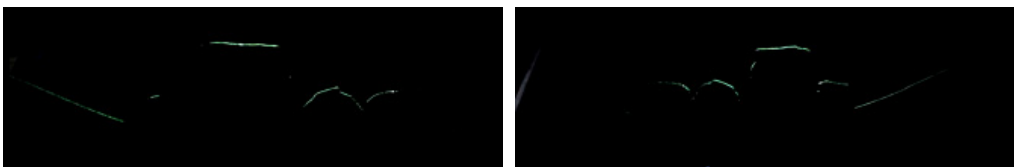
Fig. 9. Sample images of the laser lines (intersections of the laser light plane with the coal surface) from the left and right hand cameras on the basis of which the resultant image is formed
