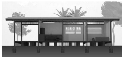
„The timber structure is self-supporting and creates pockets for the walls. The bowed butterfly roof is used for water catchment at the center of the house.” http://anmhut.com/Open-Source-House
