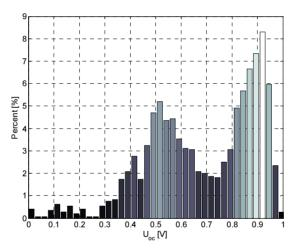
Fig. 4. The histogram of open circuit LBIC voltage  $U_{oc}(x,y)$  values obtained for the investigated solar cell.
