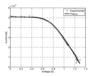
Fig. 9. The experimental data for the investigated silicon cell obtained at the maximum current point (circles) and the I–V theoretical curve calculated for parameter values obtained from the optimization process (solid line).
