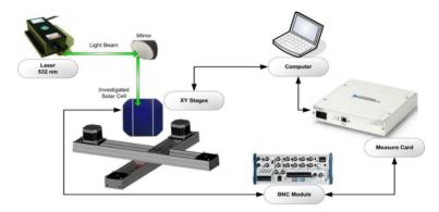
Fig. 1. The experimental set up for laser beam induced current measurements.
