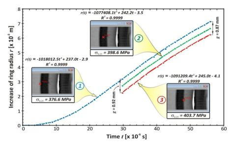
Fig. 6. The influence of position of the tracking point on the calculation of plastic flow stress of the ring material.
