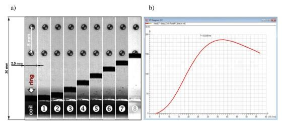
Fig. 5. The sequence of images showing the observation area with the moving ring segment (a) and the example of screen shot of the expansion velocity curve calculated from images with the use of TEMA Automotive software (b).
