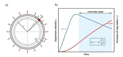
Fig. 1. Schematic illustration of ring expansion (a) and curves of radial displacement and velocity expansion (b), where  $g_o$  and g denote the initial and current width of the ring, respectively.
