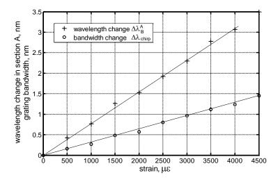
Fig. 10. Results of measurements of the sensor response to strain, obtained at a constant temperature of 25°C.
