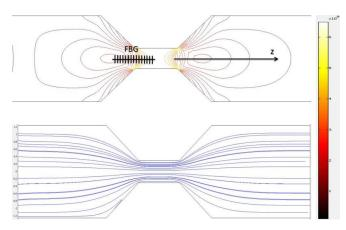
Fig. 7. Normal strain global (top) and first principal strain direction (bottom).
