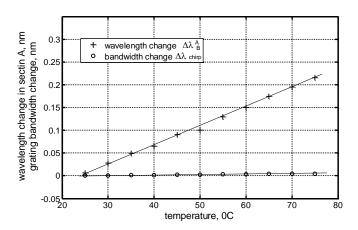
Fig. 11. The results of measurements of the sensor response to temperature, obtained at a constant strain of 1000  $\mu\epsilon$ .
