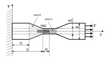
Fig. 1. Dimensions and shape of the sample used in the sensor system with a single FBG for simultaneous measurement of strain and temperature.
