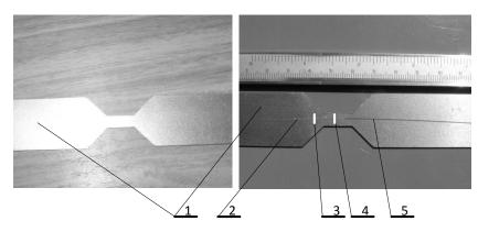
Fig. 4. The tested sensor with Fibre Bragg Grating placed on a profile sample. 1 – metal cantilever, 2. Glue joint (sikadur-30), 3-the beginning of FBG, 4 – the end of FBG, 5 – SMF28 single-mode fibre.
