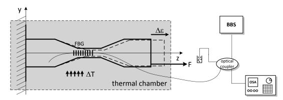
Fig. 2. Experimental system for measuring strain and temperature by means of a sensor with one FBG. BSS – broadband light source, OSA – optical spectrum analyser.
