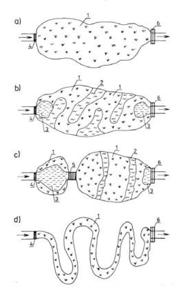
Fig. 6. Schemes of reservoirs (biofilters) for the purification of polluted water; a) one-chamber reservoir, b) reservoir with diverse surface, c) two-chamber reservoir, d) channel (ditch); 1 – surface of the reservoir covered by aquatic plants or grass, 2 – elevated areas of the reservoir or areas covered by higher vegetation, 3 – reservoir filled with water, 4 – inlet construction, 5 – rapid flow channel (cascade), 6 – outlet construction; source: CAMPBELL, OGEN [1999]
