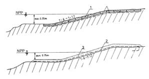
Fig. 1. Examples of a simple watering site construction: I - concrete slabs, rods or wooden boards, 2 - geotextiles,3 - sand
