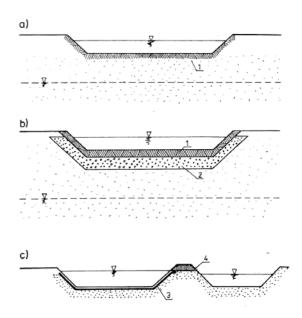
Fig. 9. Schemes of infiltration reservoirs: a) natural basin,
