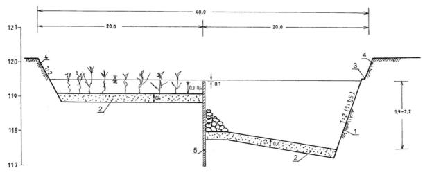
Fig. 4. A schematic cross section through the natural swimming pool; I – slope of the deep part of the pool, 2 – bottom (gravel, coarse sand), 3 – bench allowing a walk over the water table, 4 – slope covered by grass, 5 – wall separating the deep part of the pool from the shallow one
