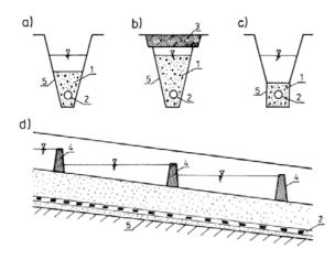
Fig. 11. Infiltration ditches scheme: a), b), c) cross sections,
