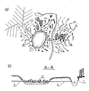
Fig. 8. A scheme of the biofilter located in the vicinity of a drainage water recipient: a) situation plan, b) A–A section; *I* – water course (drainage water recipient), 2 – dug pond covered by vegetation, 3 – outlet of the drainage water, *4* – discharge of purified water to the water course (open ditch or pipeline)
