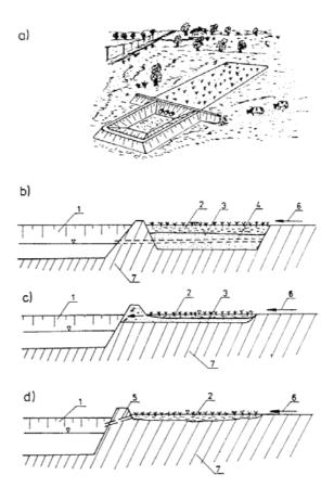
Fig. 7. A scheme of reservoir for preliminary surface runoff water purification: a) general view of the reservoir, b), c),
