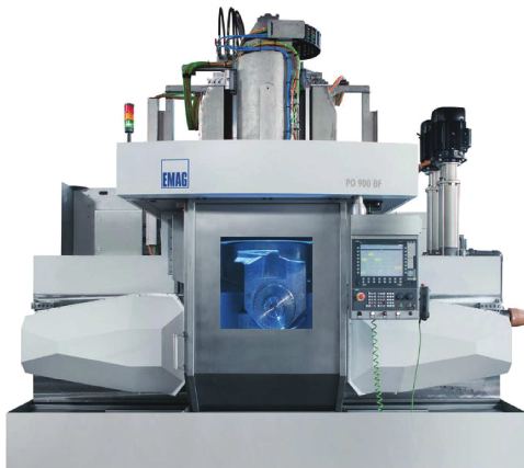
Fig. 8. The modern electrochemical machine tool EMAG PO 900 BF designed for machining the complete blisk [15].
