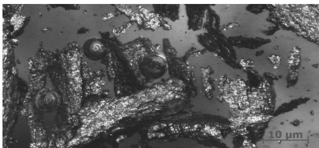
Fig. 8. Epidian 6 +IDA (80%) - Wood's alloy (20%) composite
