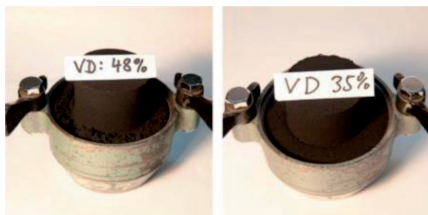
Fig. 10. Values of Georg Fischer flowability at different values of compactability of sand
