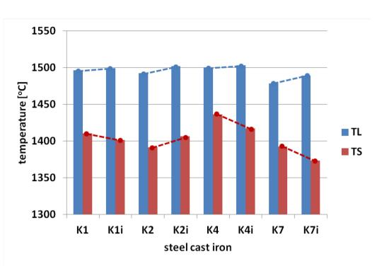
Fig. 7. Influence of cooling rate on liquidus and solidus temperature for studied low-alloyed cast steels
