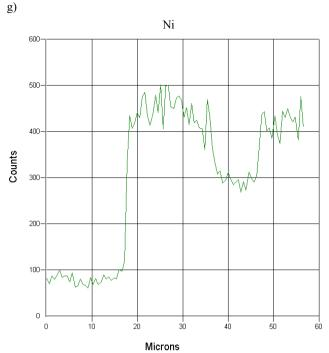
Fig. 3 (a  $\div$  g). The linear distribution of elements within the eutectic cell in pearlitic nodular cast iron with carbides containing: 3,88% C; 2,23% Si; 0,40% Mn; 1,55% Cu; 0,96% Ni; 0,99% Cr ( $C_e = 4,66\%$ )
