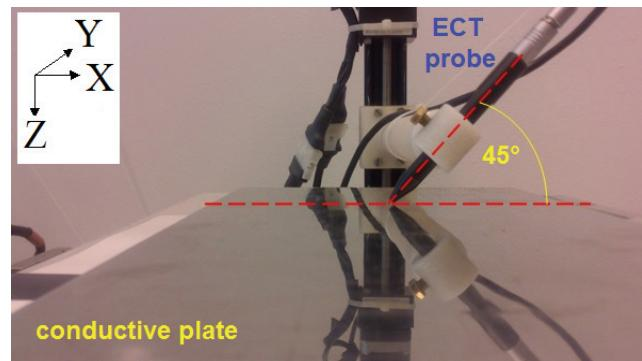
Fig. 10. Configuration of the ECT probe over the conductive specimen with defect
