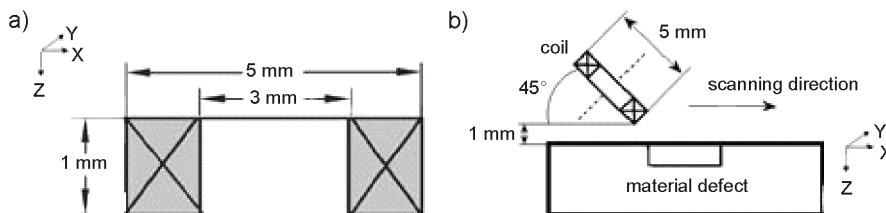
Fig. 2. A) geometry of the ECT probe, b) configuration with tilting positions
