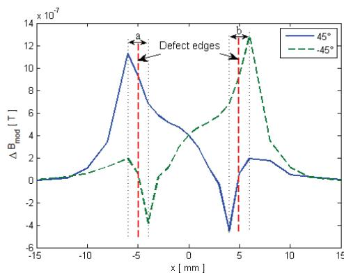
Fig. 6. Numerical simulation results: combination of differential response signals using probe tilting on 3 mm defect
