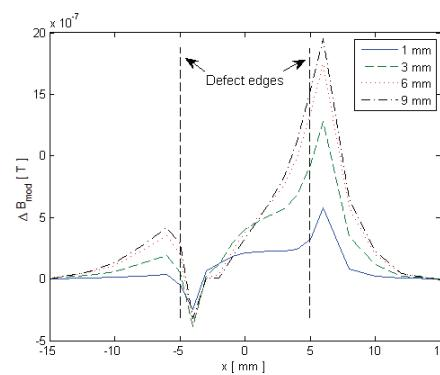
Fig. 5. Numerical simulation results: differential response signals using probe tilting, in x-axis,  $\varphi = -45^\circ$  tilt
