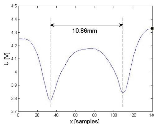
Fig. 11. Imaginary component of response signal – conventional scan
