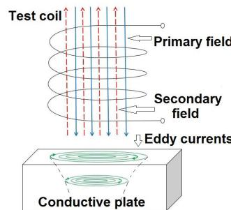
Fig. 1. Principle of the ECT method
