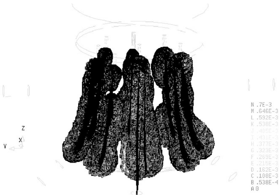
Fig. 7. The droplet dispersion (holdup) simulated by means of the cloud model, 3D picture of clouds
