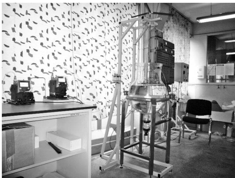
Fig. 13. The experimental setup for electrically induced extraction in a pilot scale contactor
