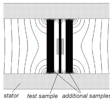
Fig. 3. Pictorial drawing of the measurement system; lines present the magnetic field distribution in the cross-section of the measurement system
