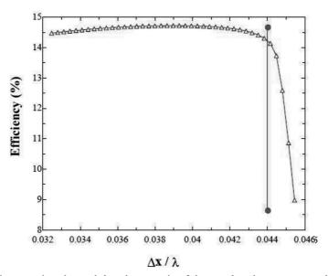
Fig. 8. Efficiency against the stack length as a ratio of the wavelength at a constant thermal input of 2000 W to the hot heat exchanger, a frequency of 398 Hz, temperature difference of 340 K and mean helium pressure of 10 bars
