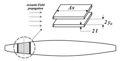
Fig. 7. Geometrical parameters of a parallel plate stack
