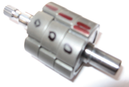
Fig. 11. Assembled rotor with 3 step-skew groups of 6 PMs
