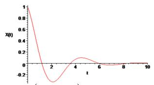
Figure 4. Transient of the error for  $\left\{\frac{c_1}{c_2} = -2, \frac{c_3}{c_2} = 3\right\} \rightarrow \{z_1 = -0.5, z_{2,3} = -0.5 \pm j1.322875656\}$ . From (107)  $\tau_1 = 2.101652954, x(\tau_1) = -0.327066$ .
