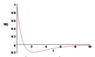
Figure 6. Transient of the error for  $\left\{\frac{c_1}{c_2} = -0.5, \frac{c_3}{c_2} = -1.5\right\} \rightarrow \{z_1 = -2, z_2 = -0.3596117969, z_3 = -1.390388203\}$ . From (107)  $\tau = 2.272247399, x(\tau_1) = -0.19366$ .
