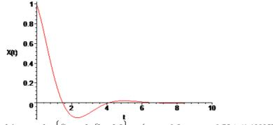
Figure 5. Transient of the error for  $\left\{\frac{c_1}{c_2} = -2, \frac{c_3}{c_2} = 2.5\right\} \rightarrow \{z_1 = -0.5, z_{2,3} = -0.75 \pm j1.19895788\}.$ From (107)  $\tau_1 = 2.32549596, x(\tau_1) = -0.151379.$
