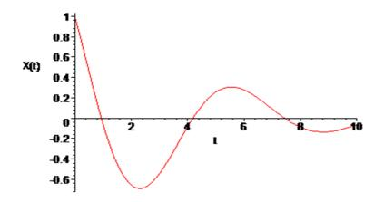
Figure 3. Transient of the error for  $\left\{\frac{c_1}{c_2} = -1, \frac{c_3}{c_2} = 0.5\right\} \rightarrow \{z_1 = -1, z_{2,3} = -0.25 \pm j0.9682458365\}$ . From (107)  $\tau_1 = 2.302983683, x(\tau_1) = -0.688656$ .
