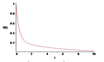
Figure 7. Transient of the error for  $\left\{\frac{c_1}{c_2} = -0.5, \frac{c_3}{c_2} = -2.5\right\} \rightarrow \{z_1 = -2, z_2 = -0.19575235, z_3 = -2.55424764\}, z_1 > z_3, \tau < 0.$
