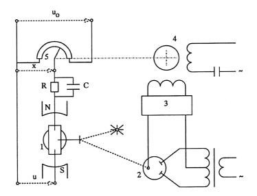
Figure 8. Voltage compensator: 1- galvanometer, 2 - photocell, 3 - amplifier, 4 - motor, 5 - potentiometer
