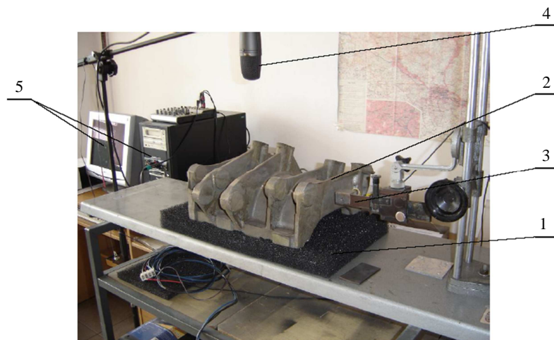
Fig. 1. General view of the test bed: 1 – measuring bench, 2 – five-rib casting from MgZA-7 magnesium alloy, 3 – device to mechanical excitation of vibrations, 4 – directional microphone to recording of acoustic field, 5 – computer with monitor to registration of sound from mixer connected to the microphone
