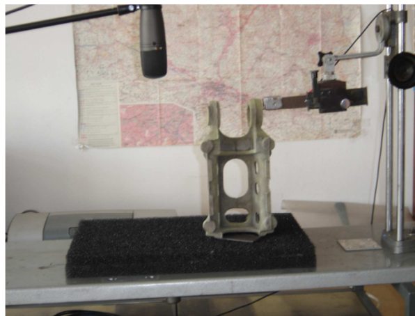
Fig. 2. The technique of fixing a 2-rib casting (the selected spot where vibrations are induced in the casting)
