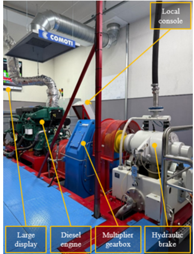
Fig. 3. The diesel engines test bench
