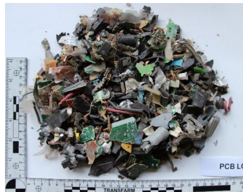
Fig. 2. LOW GRADE PCB scrap of 28 mm fraction size
