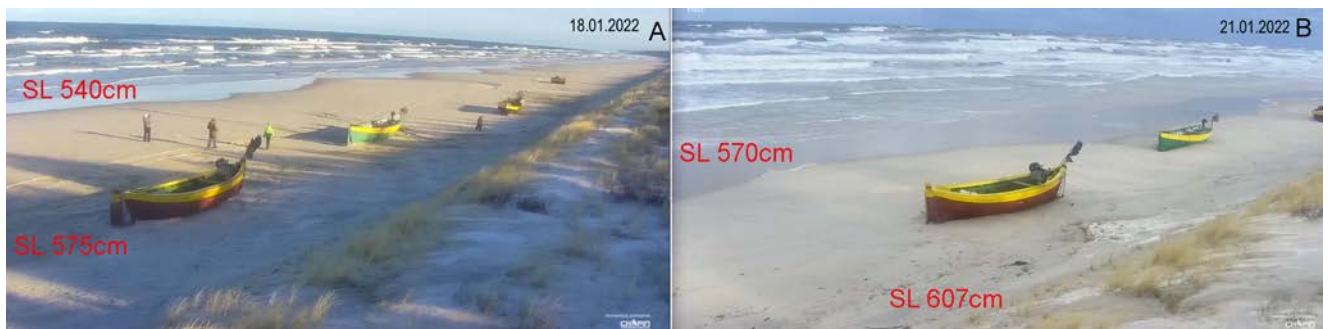
Fig. 11. Short-term sea level change vs run-up range on the beach (photos from the camera: https://nadmorski24.pl/kamery/ ). A – situation after surge Gerhild with max. SL = 575 cm. B – a situation during surge Ida II, after Ida I with max. SL = 607 cm.
