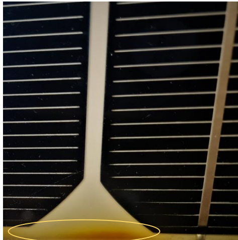
Fig. 3. Yellowing of the EVA film on the photovoltaic panel.
