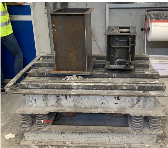
Fig. 1. Moulds on the vibrating table
