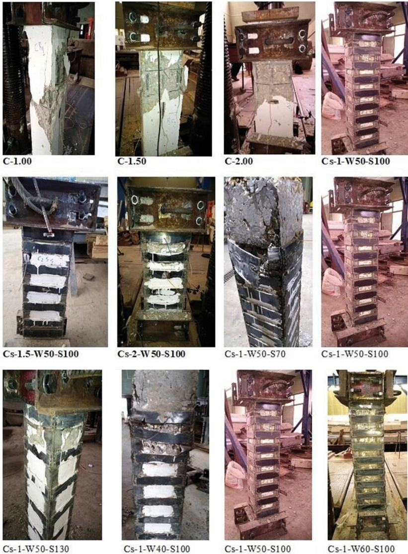
Fig. 3. Failure mechanism of specimens
