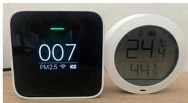
Fig. 4. Appearance of the detector, working device with a temperature and humidity sensor. Source: own
