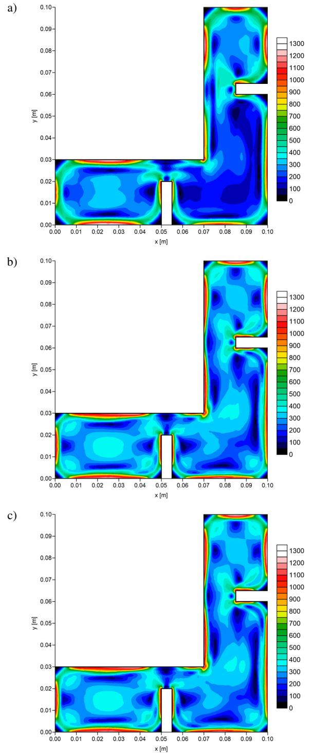
**Fig. 9.** Residual effective stresses distribution [MPa]: a) numerical model, b) RNN 2000 epochs, c) RNN 50 epochs
