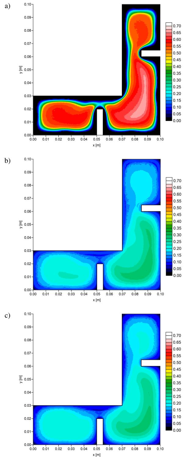
**Fig. 5.** Sum of ferrite and pearlite fraction (after cooling process): a) numerical model, b) RNN 2000 epochs, c) RNN 50 epochs
