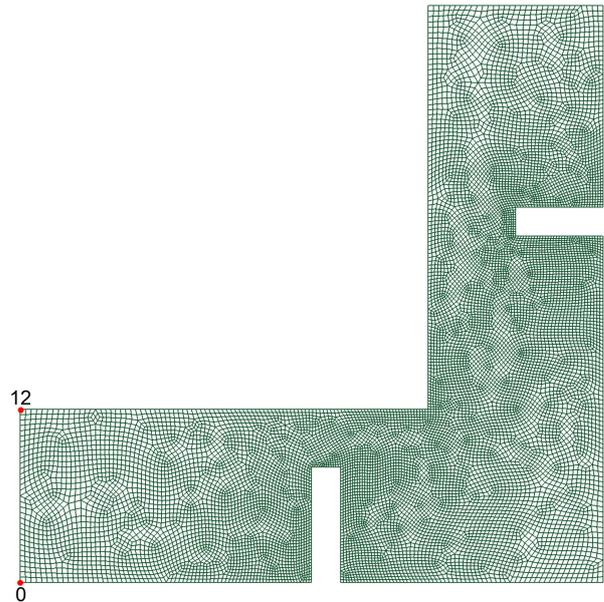
Fig. 2. Discretisation of the cross-sectional analysis space
