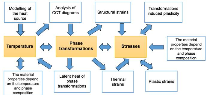
Fig. 1. Modeling scheme for heat treatment phenomena
