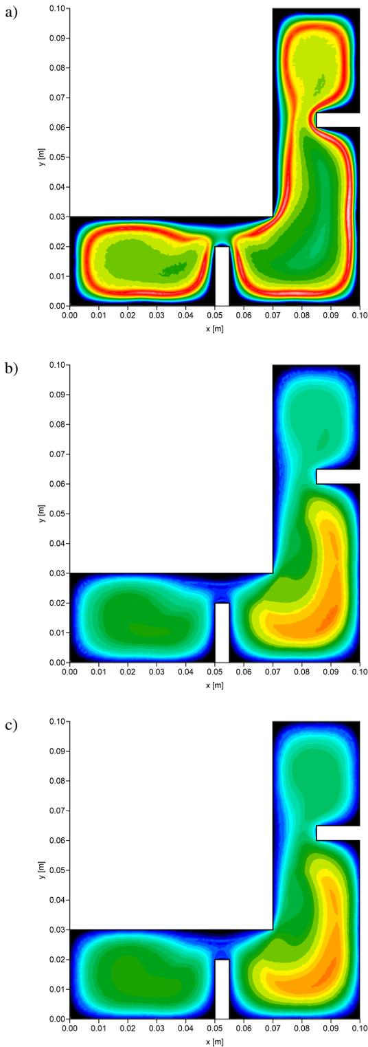
**Fig. 6.** Bainite fraction (after cooling process): a) numerical model, b) RNN 2000 epochs, c) RNN 50 epochs
