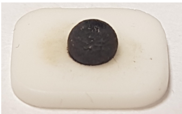
Fig. 2. Melted sample of CuSn10 tin bronze inside high temperature microscope
