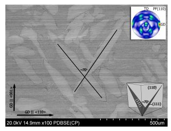
Fig. 9. Microstructure with ordered precipitations of a phase. Angular relation was marked on the unit cell and pole figure
