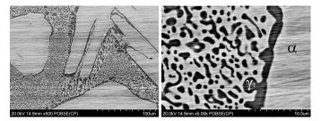
Fig. 7. Microstructure of a sample taken from zone II of DS rod; SEM observed using BSE detector; magnifications 500× and 5000×
