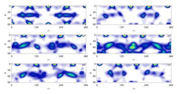
**Fig. 14.** ODF representation of orientation measured for  $\alpha$  phase in a sample from zone 3 of DS rod; it corresponds to Fig. 12
