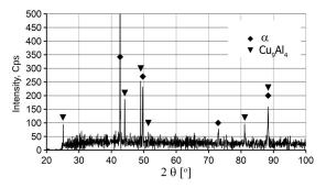
Fig. 5. Powder diffraction spectrum defining phases present in the material, Cu–Al solid solution  $\alpha$  and  $\gamma_1$  phase (Cu<sub>9</sub>Al<sub>4</sub>)
