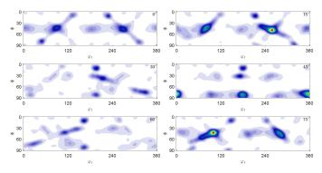
**Fig. 15.** ODF representation of orientation measured for  $\gamma_1$  phase in a sample from zone 3 of DS rod; it corresponds to Fig. 13
