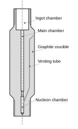
Fig. 2. Schematic illustration of a crucible used in the experiment
