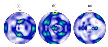
**Fig. 12.** Pole figures of sample from zone 3 of DS rod measured for  $\alpha$  phase at three crystallographic planes {100}, {110}, {111} and recalculated in MTEX toolbox for Matlab
