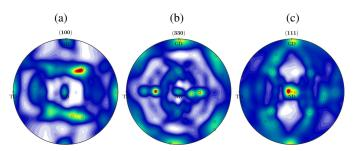
**Fig. 13.** Pole figures of sample from zone 3 of DS rod measured for  $\gamma_1$  phase at three crystallographic planes {100}, {330}, {111} and recalculated in MTEX toolbox for Matlab
