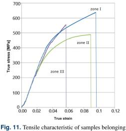
Fig. 11. Tensile characteristic of samples belonging to three zones of a DS rod
