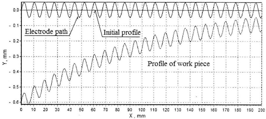
Fig. 7. The effect of vibration of tool on final profile ( $R_0=10$  mm,  $a_o=0.6$  mm,  $v=0.3$ )
