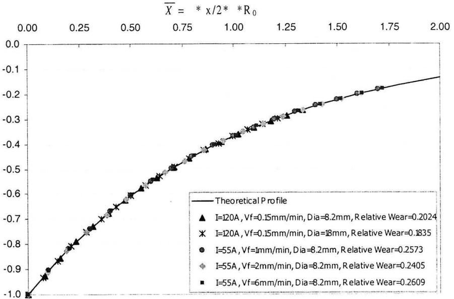
Fig. 9. Comparison of theoretical and experimental results in non-dimensional system coordinates.
