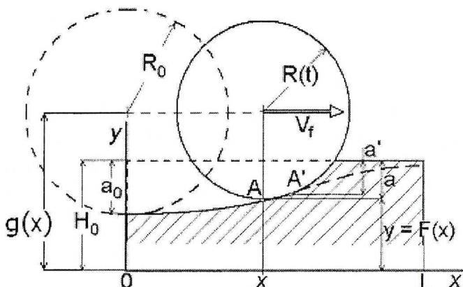
Fig. 3. Scheme of machining of flat surface using rotating tool
