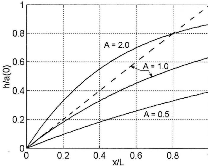
Fig. 4. Profile of machined surface at different values of  $A$
