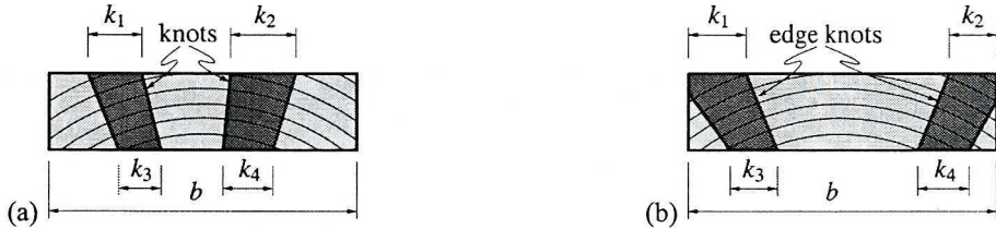
Fig. 9. Cross-section of a board (a) without edge knots, (b) with edge knots
