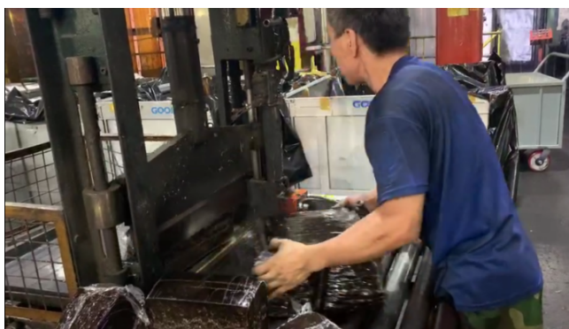
Fig. 1. Specified weight cutting of irregular rubber realized by worker's experience
