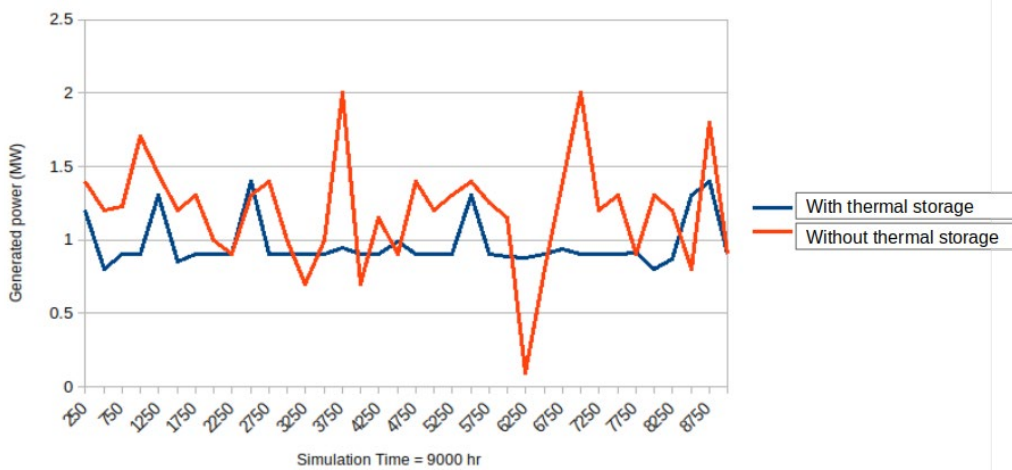
Fig. 10. A comparison of power generation with and without the use of a thermal storage system [MW]
