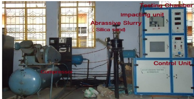
Fig. 2. Set up for Erosion Test
