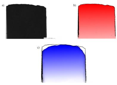
Fig. 6. Top view of the tip visualized with a) an optical measuring machine, b) microCT and c) the CS3600 camera. Black line in b) and c) the edge of the image obtained with the optical machine in a). The blank in b) and c), corresponds to the difference between the optical measuring machine edge and the 3D image scanned with microCT and the IOS and represents loss of information.
