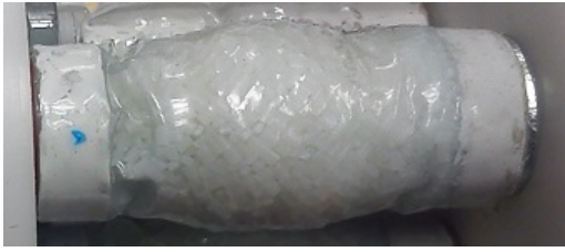
Fig. 4. VPP damper filled with polystyrene
