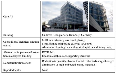
Fig. 1. Unconventional façade technology for dematerialization. Unilever Headquarters, Hamburg, Germany
