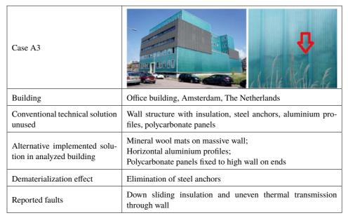
Fig. 3. Unconventional façade technology for dematerialization. Office building, Amsterdam
