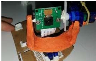
Fig. 12. Mechanism for mimicking head movement created with the 3D pen
